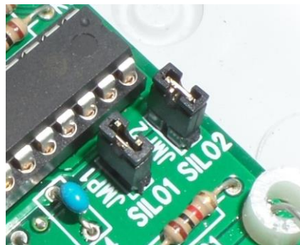
Photo 10: Both silos are connected
